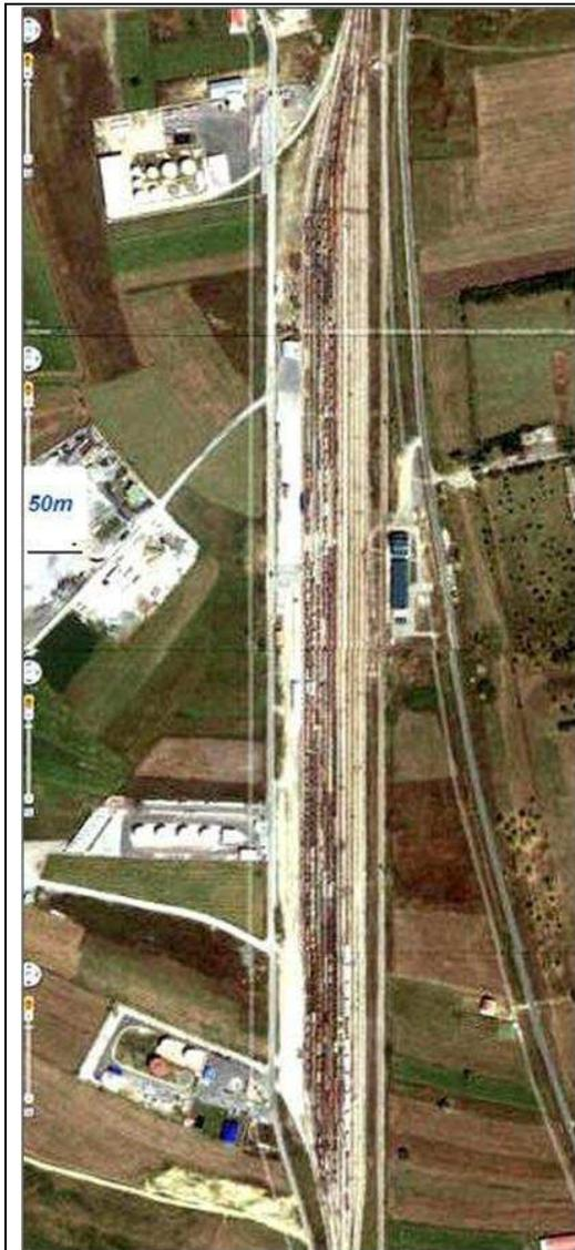
The terminal is a typical station of shunters for conventional railway wagons, which can also operate with containers.
